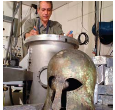
▲ Greek bronze helmet, 7th century BC, property of The Manchester Museum, being prepared for non-destructive neutron analysis as part of an investigation into its structure and metallurgy (photo STFC)
